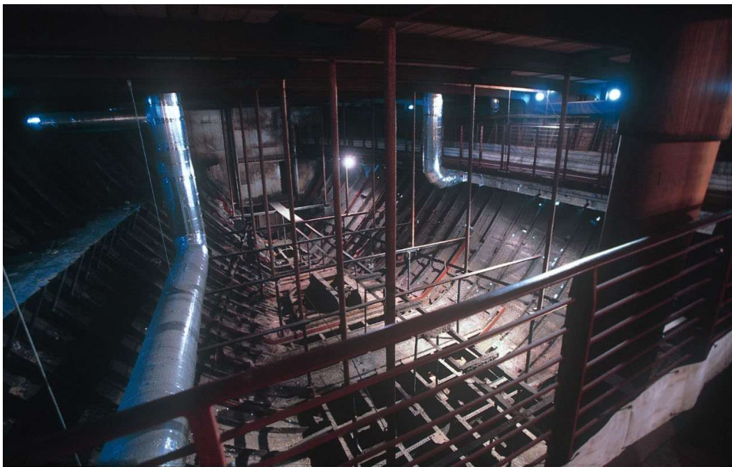
Figure 2: Interior of lower ship's hull, showing iron structure and desiccated air delivery ducts.
