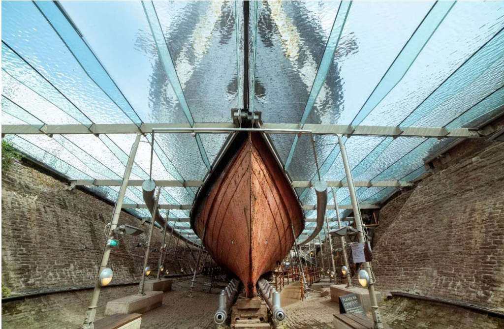
Figure 1: The glass plate creates a seal around the hull below the waterline. Ducts and vents are positioned to create a layer of dried air adjacent to the historic iron.
