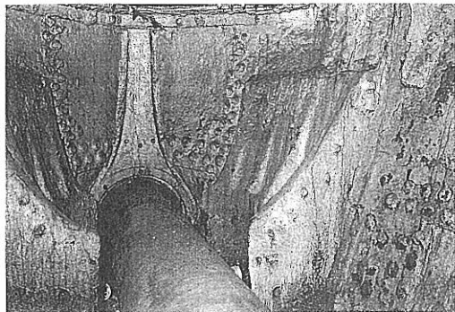
[53] Surviving detail from the first phase. The stuffing box, a substantial iron casting where the screw shaft entered the stern of the ship.
