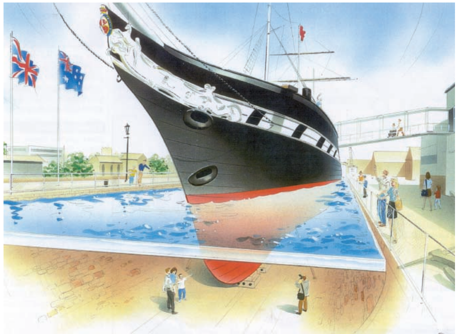
Figure 8 Artists impression of the controlled space around the lower hull of the ss Great Britain.
