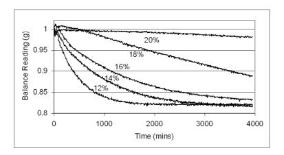
Figure 2 Desiccation - recorded as weight loss - from a range of FeCl<sub>2</sub>·4H<sub>2</sub>O (1.0000 g) samples run at different levels of RH.
