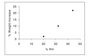
**Figure 1** Weight increases for iron/FeCl<sub>2</sub>·4H<sub>2</sub>O mixtures at varying RH (after Turgoose [9]).
