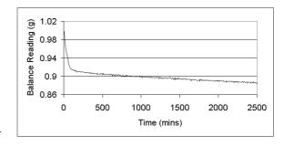
Figure 7 β-FeOOH equilibrated to 41% RH and exposed to 19% RH for 2500 minutes.
