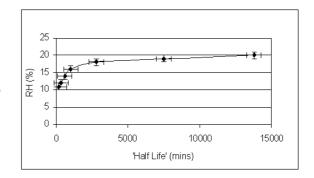
**Figure 4** The relationship between half-life of partially desiccated FeCl $_2$ '4H $_2$ O and RH.
