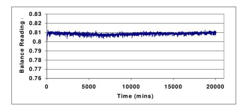
Figure 5 The behaviour of 0.31 g ferrous chloride dihydrate mixed with 0.50 g iron powder at 19% RH for two weeks. No change in micro/ macroscopic appearance (corrosion) of the mixture was observed between the start and the end of this test.
