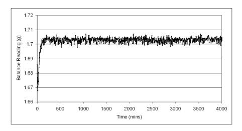
Figure 8 β-FeOOH equilibrated to 41% RH and exposed to 80% RH for 4000 minutes
