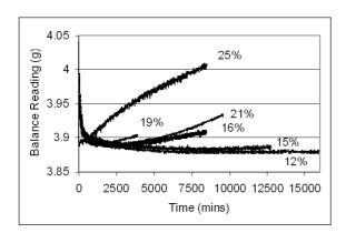
Figure 9 Weight changes of β-FeOOH /iron mixtures at 12%, 15%, 16%, 19%, 21%, 25% RH, All tests were conducted with 2,00 a of bFeOOH mixed with 2 g of iron powder.
