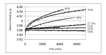
Figure 6 Corrosion of iron in the presence of ferrous chloride tetra-hydrate at fixed RH values. All tests were conducted with 2.0 g of FeCl<sub>2</sub>·4H<sub>2</sub>O mixed with 2.0 g of iron powder.
