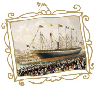
**At 98 metres, the SS Great Britain was the longest passenger ship in the world from 1843 to 1854. She was also the first screw-propelled, ocean-going, iron hulled steam ship.**
