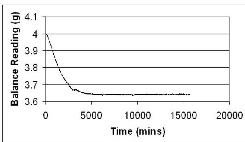
**Figure 4** FeCl<sub>2</sub>.4H<sub>2</sub>O mixed with an equal mass of iron powder and sequentially subjected to 48 hrs at 15% relative humidity followed by 6 hrs 22% relative humidity at 20°C.
