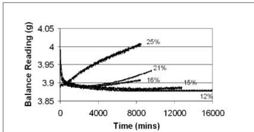
**Figure 3** Response of samples comprising equal masses of iron powder and  $\beta$ -FeOOH to different fixed relative humidity values at  $20^\circ\text{C}$ .<sup>11</sup>
