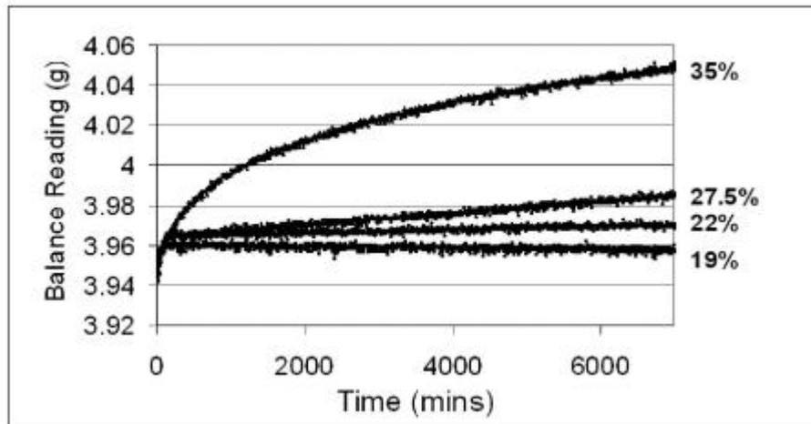
**Figure 2** The response of samples comprising equal masses of iron powder and  $\text{FeCl}_2 \cdot 4\text{H}_2\text{O}$  to different fixed relative humidity values at  $20^\circ\text{C}$ .<sup>11</sup>
